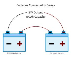
A Series connection will double VOLTAGE while AMP HOURS remain constant.
