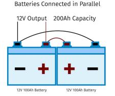
A Parallel connection will double AMP HOURS while VOLTAGE remains constant.
